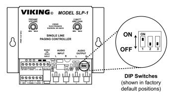
Note: Place DIP switches in the desired position then momentarily power down the unit.
