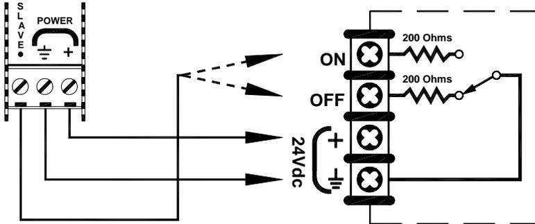
Functional Equivalent to Internal Solid State Switching Circuit
