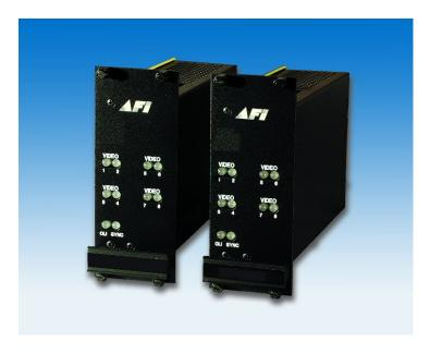
The American Fibertek 980 Series transmits eight channels of high-quality 10 bit digitized video on one multimode optical fiber. Designed to be completely transparent to all camera and monitor manufacturers, this system requires no field adjustments at installation or additional maintenance thereafter. Diagnostic indicators provide a quick visual indication of system status. The "Afinety" intelligent remote monitoring system is available on this product, please consult factory.
