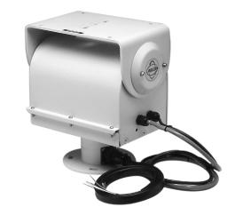
The **PT680-24P** is a medium duty outdoor pan/tilt designed to accept a maximum load of 50 pounds (22.7 kg). The unit is factory prewired for feedthrough of the motorized zoom lens, camera power, enclosure power, and video signals. All connections are made at the input connector, eliminating the need for wiring harnesses made in the field. This feature greatly reduces installation time, while increasing the reliability and serviceability of the system.
