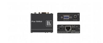
The PT-110EDID is a twisted pair transmitter for computer graphics video signals. It converts a computer graphics signal into a twisted pair signal that is converted back to a computer graphics video signal when used with a compatible receiver.
