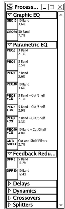
The primary interface for the P4800 is a Windows-based software program that mimics the functional block diagrams used in sound system design. Unlike many other DSP products that constrict design freedom with preset templates, the processing blocks in the P4800 can be applied in any order, to any input or output. Processing blocks can be copied and pasted to duplicate processors across multiple channels. They can also be linked for more efficient stereo or global control.
