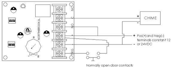
For this application Switch #1 and Switch #4 should be in the OFF position.
