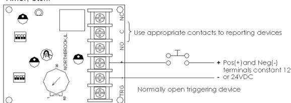
For this application Switch #1 should be in the ON position and Switch #4 is not used in this application.
