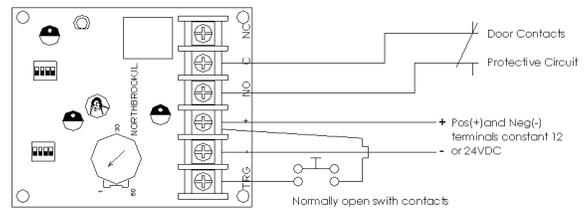
For this application Switch #1 should be in the OFF position and Switch #4 should be in the ON position.
