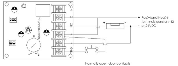
For this application Switch #1 should be in the OFF position and Switch #4 should be in the ON position.
