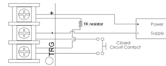
For this application a 1K (1,000 ohm) resistor must be installed as shown. (resistor not supplied)
