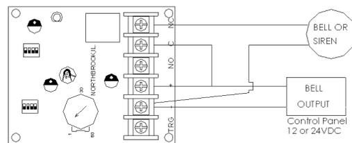
For this application Switch #1 should be in the ON position and Switch #4 is not used in this application.
