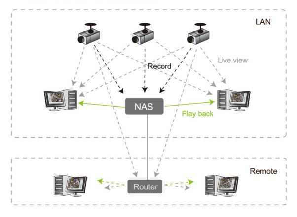
Cameras provide the live video streams to users directly, not through the NAS
