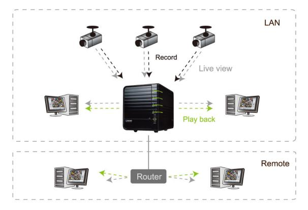
NAS directly connects to cameras. Users access NAS to receive the live streams
