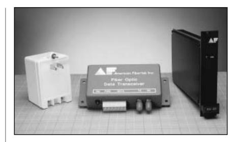
The American Fibertek 03 Series transmits and receives high-quality, RS232 data on dual multimode optical fiber. Designed for continuous long-range, interference free data transmission, these systems require no field adjustments at installation or additional maintenance thereafter. Diagnostic indicators provide a quick visual indication of system status. Equipment may be ordered as stand alone modules or rack cards that are mounted in the American Fibertek Card Cages: SR-20/2 or SR-20R/1.
