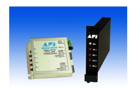
The American Fibertek 480 Series transmits and receives one simultaneous channel of data over a single singlemode optical fiber. The system is comprised of two transceivers forming a point-to-point communications link. The system is designed to be completely transparent to data protocol and can be configured as RS-485 (2 wire or 4 wire), RS-422, RS-232 or Manchester Code. For ease of installation, diagnostic indicators provide a quick visual indication of system status.
