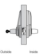
Lever handles are Free Wheeling in locked position. Shaded area denotes Free Wheeling lever.
