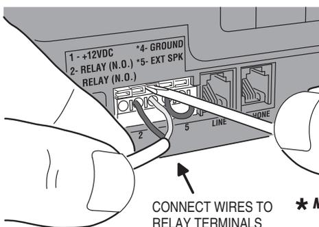
USE A SMALL SCREWDRIVER TO PUSH ON THE TERMINAL LOCKS TO ALLOW THE WIRE TO SLIDE INTO THE TERMINAL HOLE
