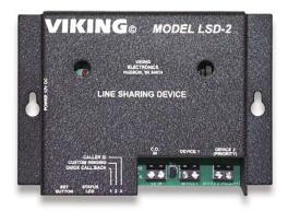
For incoming calls, the LSD-2 can route calls to the DEVICE 2 (PRIORITY) port using Caller ID, Distinctive Ring, or Quick Call Back. All other calls will be routed to the **DEVICE 1**. Alternatively, the **LSD-**2 can be set up so that all inbound calls are routed to the DEVICE 2 (PRIORITY) port. Note: Caller ID is not passed through the LSD-2 to the devices.
