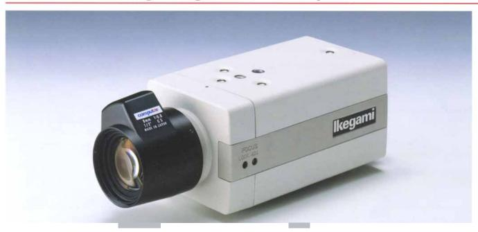
ICD-47(EIA)/47E(CCIR) is a high-sensitivity, higher-resolution B/W surveillance camera with 1/2"CCD for high-quality pictures. The camera incorporates Line-Lock, Auto Shutter, Back-light compensation, two way Auto Iris and delivers horizontal resolution of 570TV lines(EIA)/560TV lines(CCIR) with Minimum Illumination of 0.02 Ix/f1.4. Smear Level -120dB. The camera also supports near infrared imaging.
