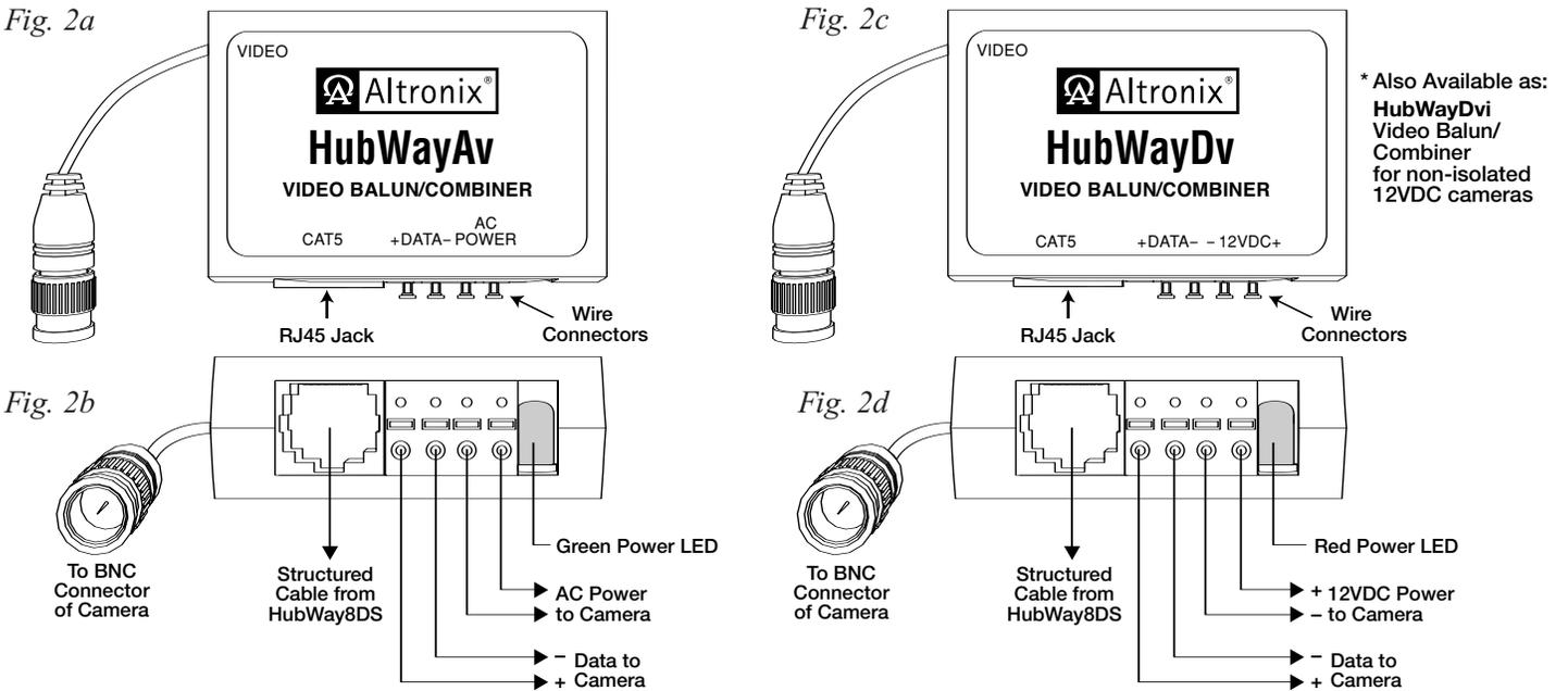
HubWayAv passes AC voltage from pins 4, 5, 7, 8 to terminals marked [AC Power] (Fig. 3, pg. 5).
