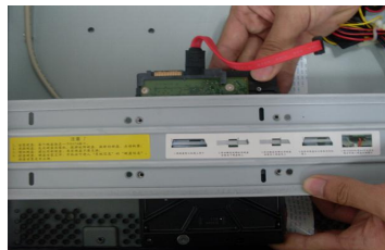
Align the HDD with the holes provided on the HDD bracket.
