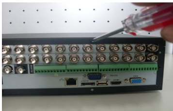
Remove the top cover from the DVR.
