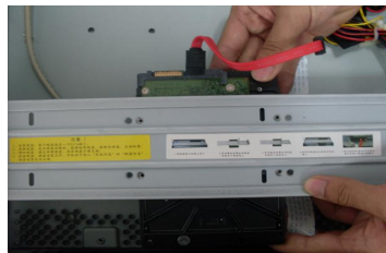
Align the HDD with the holes provided on the HDD bracket.
