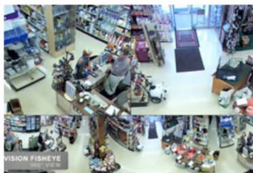
Dewarped Image: 2 PTZ views & 1 360 degree view
