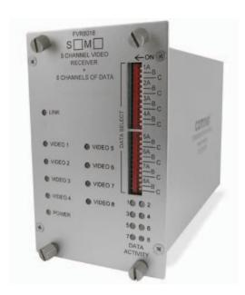
8-channel digital video + 8 bi-directional data channels + 10-bit digital short-haul video
