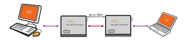
RJ45 patch lead (depends on attached device) Multimode or singlemode fiber
