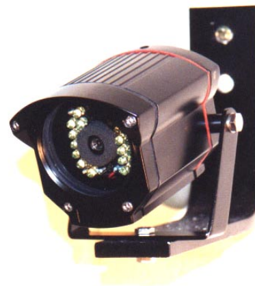
Above: The EX25N.8306 is a combined camera + infrared illuminator comprised of an IR-Optimized S300 CCD sensor and 24 LEDs. It is an excellent 24-hour camera for short-range video from 6 to 40 feet.
