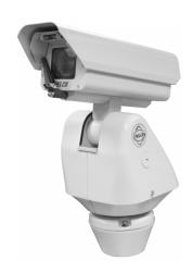
A powder-coated, aluminum construction makes the **ES30PC** and **ES31PC** ideal for either indoor or outdoor applications. The system has an absolute operating temperature range of -50° to 140°F (-45° to 50°C). Within two hours after power-up, the entire unit can de-ice and be operational from a temperature of -13°F (-25°C).
