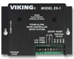
The **ES-1** is a door controller designed to operate a door strike or magnetic lock upon receiving a valid card read and/or keyless entry code from Wiegand devices. One **ES-1**, one or two Wiegand devices and a door strike or magnetic lock of your choice is required for each entry point.
