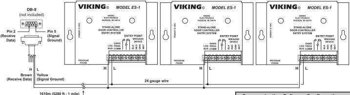
If the RS-232 input of a PC, printer, etc. is capable of receiving TTL level RS-232 signals, then the **LOG BUS** can be wired directly into the RS-232 "Receive Data" and "Signal Ground" pins to receive ASCII data. Windows "Hyper-Terminal" can be used to receive the data on a PC. Use the settings in the chart at the right:
