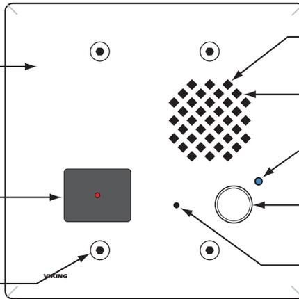
**Speaker Screen:** Stainless steel speaker screen with 0.018" diameter holes to prevent punctures from paperclips, etc.
