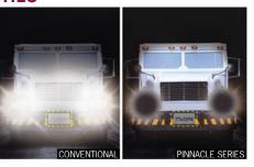
The Pinnacle Series is equipped with HLC (Highlight Compensation) function which effectively inverts strong lights (such as car headlights) to provide clearer images and increases brightness level of the rest of the image which on a typical CCD camera would be darkened to compensate for bright spots (BLC function)
