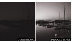
The minimum illumination level of Polaris Vision 2 cameras is down to 0.00004Lux which enables users to get recognizable images under extreme low light conditions. Combined with advanced digital noise reduction (3D-DNR) technology images are clear and in-focus.
