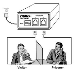
For prison applications, the DLE-200B saves the need for dedicated phone lines. Prisoners can converse with visitors phone to phone without dial tone or ringing. Note: Internal dipswitch 1 must be ON, enabling the ring down and dial tone off mode (see Programming section B).
