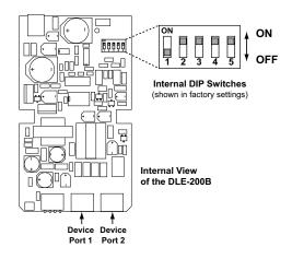
**Important:** The **DLE-200B** components are sensitive to static electricity. Personnel and the work area should be grounded before handling.
