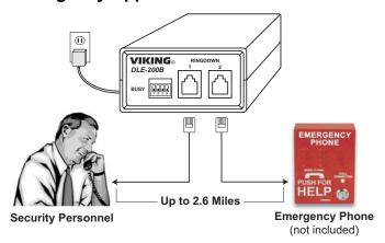
When used with emergency phones, the DLE-200B saves the expense of dedicated phone lines. When the button on the emergency phone is pushed, the DLE-200B will provide ringing to a security phone.
