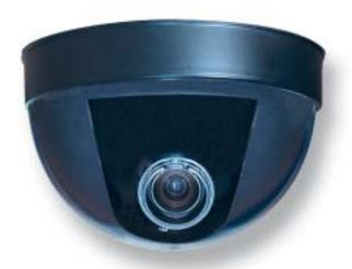
Our 1/4" color varifocal dome camera features an adjustable 4-9mm lens with a built-in electronic shutter. The camera can rotate 360 degrees. It has a .92 lux with 420 line resolution and a 12V DC power supply is included. A B/W version of this camera can be found under model number CVC-1805DC.
