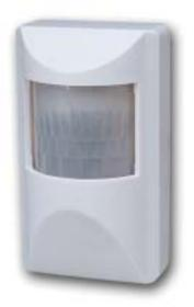
Our 1/3" B/W CCD camera is encased in a white PIR housing. It has a .5 lux sensitivity with 420 line resolution. It features a 3.6mm wide angle pinhole lens and built-in electronic shutter. A 12V DC power supply is included. A color version of this camera can be found under model number CVC-565PIR and CVC-572PIR (with working PIR). A fully adjustable wall/ceiling mount is included with this unit.
