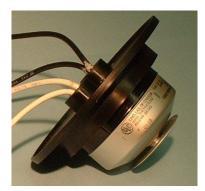
Spec. Sheet #2 Modified Pigtail (MP) Detector The THERMOFLEX® product group includes standard detectors that have the additional feature of terminal protection from water and condensation. Each MP detector is available in single or multiple circuits with Normally Open and/or Normally Closed contact configurations, and any of the fixed temperature settings including 135°, 165°, 200° and 285° F.
