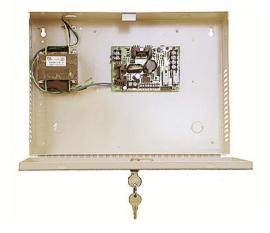
12/24 VDC, 6 amp switching power supply is agency listed for access control (UL 294 and CSA Certified). Features include field selectable voltage, Form "C" relay fault reporting, visual fault indication and an additional output for Fire Alarm Interface (FAI). Systems integration applications include system power, door strikes, mag locks, card readers and fire alarm interface for emergency exit.
