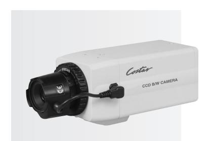
The CCM3600N is a 1/3" CCD black-and-white camera with 600 lines of resolution and a low light sensitivity of 0.1 lux at F1.2 sensitivity. With advanced controls for BLC, AGC and Gamma, the CCM3600 provides superior high-resolution image quality for a variety of applications. This compact professional surveillance camera features a C/CS/back-focus ring and a terminal strip for easier installation. The CCM3600N provides easy connection for video or DC lenses with a 4-pin connector.
