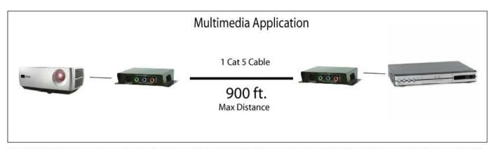
The Cyrex CCVB offers a convenient and cost effective solution to transmitting Component Video over 4 pairs of CAT5 unshielded twisted pair (UTP) cables. Maximum distance up to 900ft. Supported resolution - 480I /480p/720p/1080i
