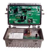
The LPA-860-36G is a two-way CATV line extender amplifier designed for outdoor applications. The amplifier has a forward bandwidth of 53-860 MHz and a reverse bandwidth of 5-42 MHz. The LPA-860-36G contains GaAs hybrid modules ensuring high forward output levels with very low distortion.
