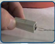
Remove 1/4" of wire insulation from the UTP wire.
