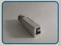
Position the BL3725 with the UTP connector side facing you.
