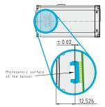
The back focal length on each camera is carefully measured and adjusted by our patented "CSAT" procedure. This guarantees an optimum distance between the lens flange and the sensor and ensures outstanding image quality based on compliance with optics standards.
