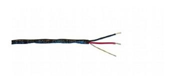
Kramer's BCP-1T is a high-quality, plenum rated, shielded pair style cable that routes balanced mono or unbalanced stereo audio signals in professional AV systems. It is also ideal for any application where a low capacitance 22 gauge shielded pair is appropriate including control panels for Sierra Video matrix switchers.
