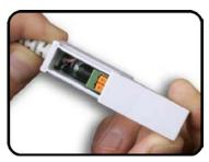
Slide off cover, raise orange IDC connectors and insert wires.
