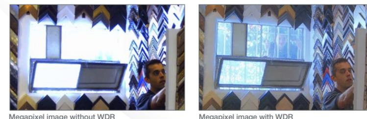
Users can achieve clear images in extreme lighting conditions with MegaVideo® Compact WDR cameras in resolutions of 1080p and 3MP. Wide Dynamic Range up to 100dB at full resolution balances light and dark areas in the same scene, such as in the lobby of an office building, the loading dock at a distribution facility or many retail environments.
