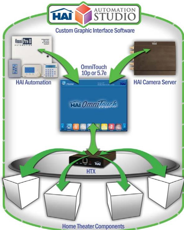
The HTX works with HAI's IP-based Touchscreens, such as the OmniTouch 10p and 5.7e, to control your home theater equipment. HTX configuration requires HAI Automation Studio software (HAI Part Number 1126) which is also used to develop the Touchscreen's custom graphic interface.
