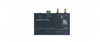
The 705xl is a twisted pair transmitter for composite video signals. The 705xl converts a composite video signal to two twisted pair signals and the 706xl receiver converts the twisted pair signals back into two composite video signals.
