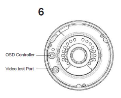
Set the desired OSD feature by using the OSD controller. (Refer the SOD manual to set up the desired OSD) in case of a installer has portable monitor, connect the video jack to the video test port to set up the OSD.
