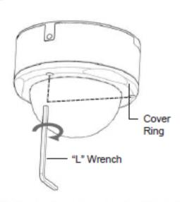
Tighten the screw by using the "L"wrench and complete the installation.
