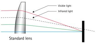
The problem can be rectified by using IR-corrected lens, which focuses both the visible and the infrared light in the same vertical plane.
