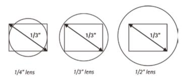
When replacing a lens on a megapixel camera, a high quality lens is required since megapixel sensors have pixels that are much smaller than those on a VGA sensor (640x480 pixels). It is best to match the lens resolution to the camera resolution in order to fully use the camera's capability.
