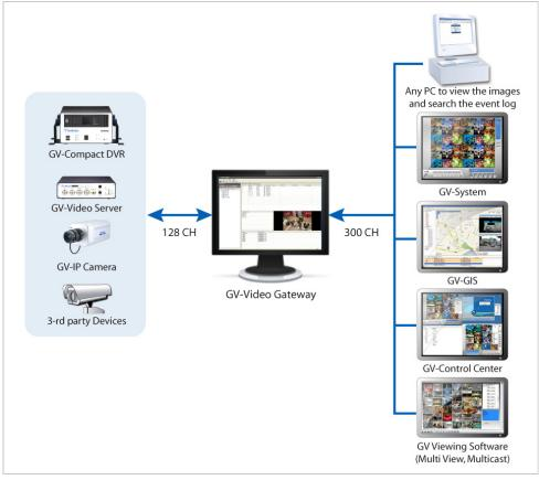
**Note:** The arrows in the diagram indicate the direction of the connections.
