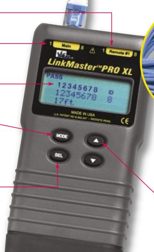
JEW – Using the cable capacitance method, length is displayed automatically if there is no splits or shorts in the Cable Test mode. If a remote is present in the Length mode, the ID number will be displayed. The length of individual pairs can be measured, and cross-over and reversed pinned cables are recognized when using Length mode.
