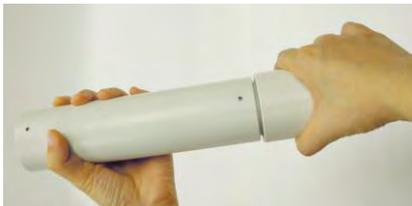
6. Thread the wires and cables through the tube, assemble the tube to the box cover and tighten the torxes with the supplied torx wrench (GV-Mount100, No. 7).
