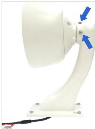
4. Thread the camera cable and secure the pendant tube to the plates. Slide the 30 mm M8 screws (GV-Mount903, No. 2) from the front and secure from the backside using plain washer (GV-Mount903, No. 3), split washer (GV-Mount903, No. 4) and secure with M8 screw cap (GV-Mount903, No. 5).
