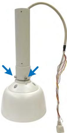
4. Thread the camera cable through the box cover (GV-Mount100, No. 2), assemble the box cover and the tube, and tighten the torxes with the supplied torx wrench (GV-Mount100, No. 7).
