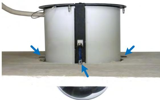
6. Put on the in-ceiling cover (GV-Mount907, No. 9) to finish installation.
