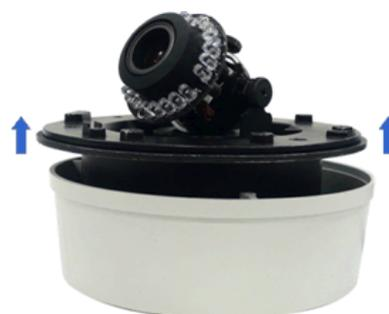
B. Secure the back cover to the wall mount bracket from the interior with M5 screws (GV-Mount900, No. 4).
