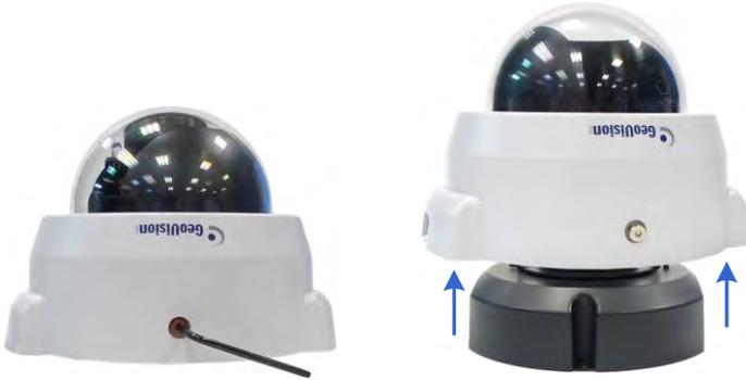
5. Align and secure the camera body to the wall mount bracket with three M3 screws (GV-Mount909, No. 4).
