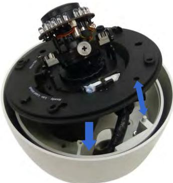
5. Thread the cable through the housing cap (GV-Mount901, No. 2) and secure with M6 screws (GV-Mount901, No. 4).
