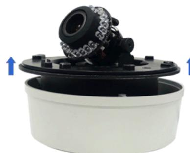
B. Secure the back cover to the wall mount bracket with M5 screws (GV-Mount900 for GV-VD Series, No. 4).
