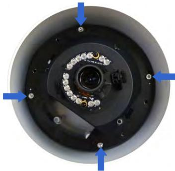
4. Secure the housing cap and the dome housing with M6 screws (GV-Mount902, No. 4).
