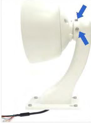
4. Thread the camera cable through the mounting bracket and secure the pendant tube to the bracket. Slide the 30 mm M8 screws (GV-Mount400 / GV-Mount410, No. 3) from the front and secure from the backside using plain washer (GV-Mount400 / GV-Mount410, No. 5), split washer (GV-Mount400 / GV-Mount410, No. 6) and screw cap (GV-Mount400 / GV-Mount410, No. 7).
