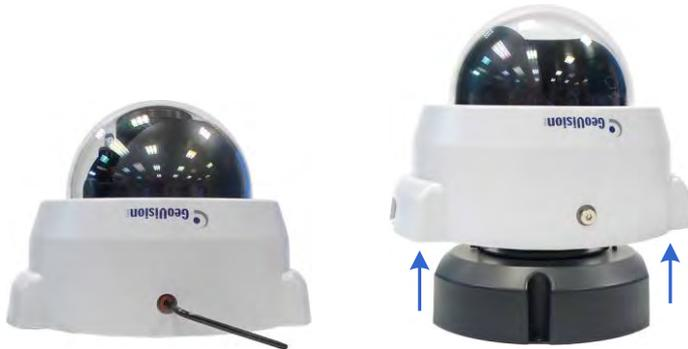
3. Secure the camera to the mounting plate with M3 screws (GV-Mount913, No. 2). Use the holes indicated with “FD” to help you align the camera.
