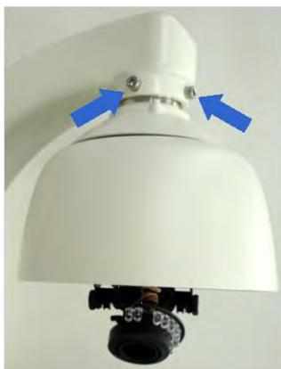
9. Conceal the junction box with M5 screws using the torx wrench (GV-Mount203, No. 5).
