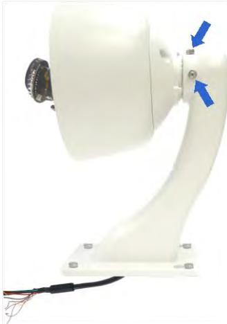
6. Thread the camera cable through the mounting bracket and secure the pendant tube to the mounting bracket. Slide the 30 mm M8 screws (GV-Mount400 / GV-Mount410, No. 3) from the front and secure from the backside using plain washer (GV-Mount400 / GV-Mount410, No. 5), split washer (GV-Mount400 / GV-Mount410, No. 6) and screw cap (GV-Mount400 / GV-Mount410, No. 7).
