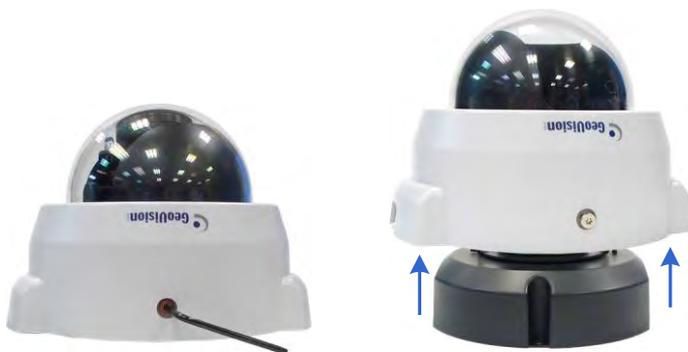
2. Secure the camera body to the housing plate (GV-Mount902, No. 6) with 3 small screws (GV-Mount902, No. 7).
