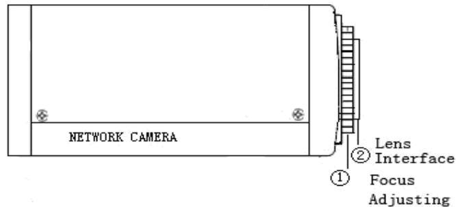
Fig 2.1.1 Side Elevation of DS-2CD832F(-E) network camera
