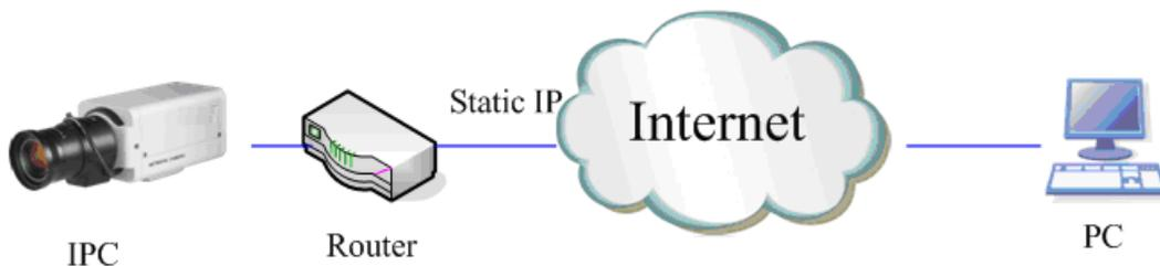
Fig.3.6.1 Static IP through Router access IPC
