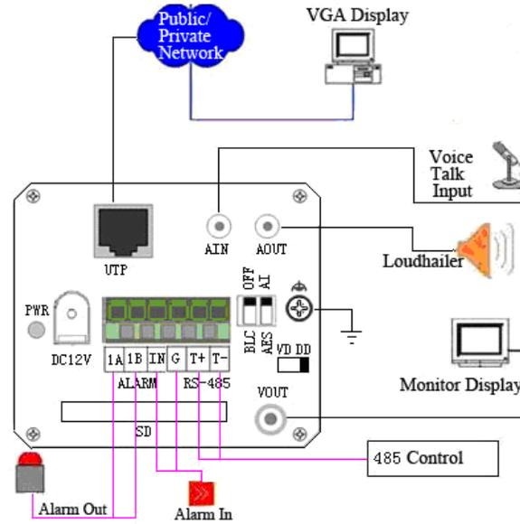
Fig 2.2.11 Topological Graph of Network Camera
