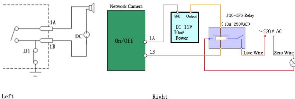
Fig 2.1.12 Alarm output
