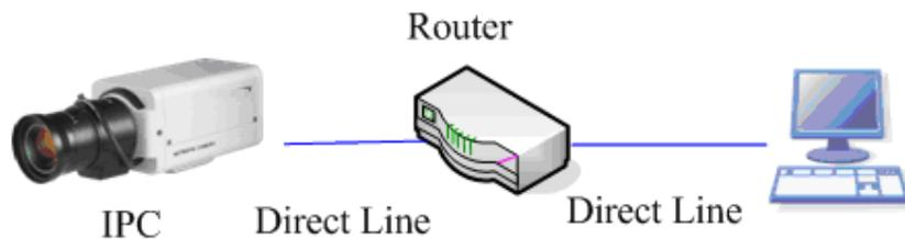
Fig. 3.1.4 Direct Line Connection
