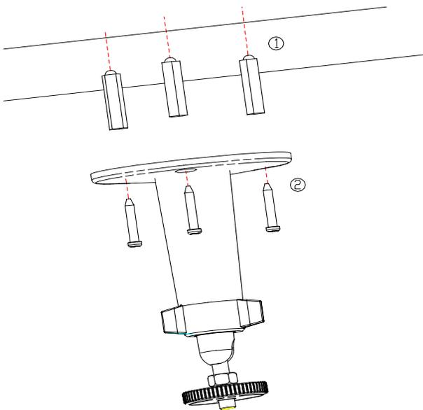
Fig 2.2.1 Fix Ceiling Bracket
