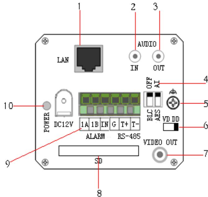
Fig. 2.1.5 Rear Panel of DS-2CD802, DS-2CD812, DS-2CD892 series
