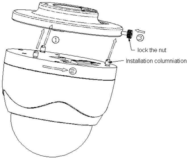
Fig 2.2.6 Dome camera fixing
