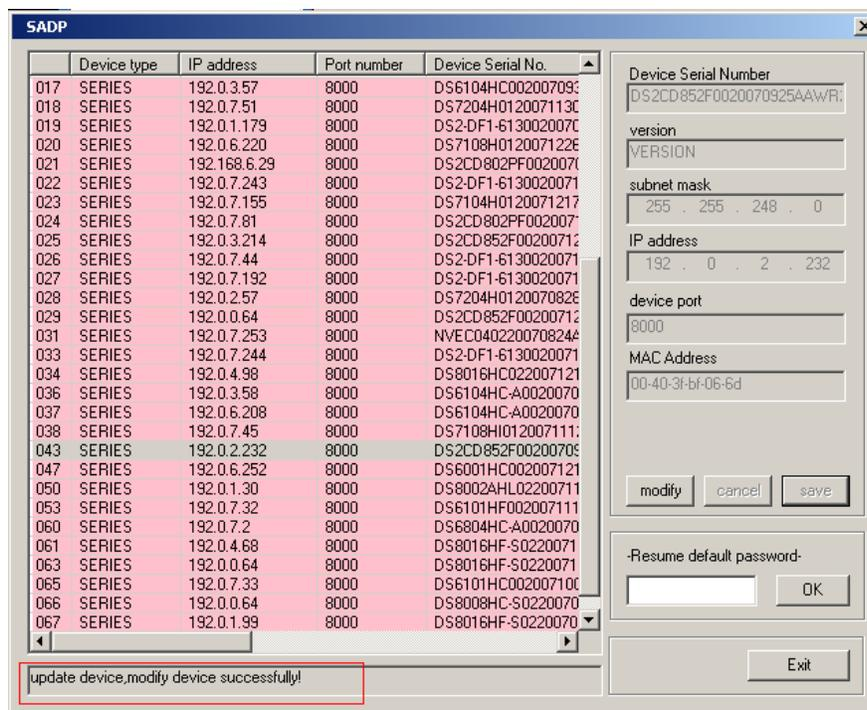
Input the new IP address, subnet mask, and port number, and click 'save' button. If a dialog pops up, showing 'saved successfully', that means you have modified the configuration information; if 'saving failed' dialog pops up, click the 'cancel' button to quit it.
