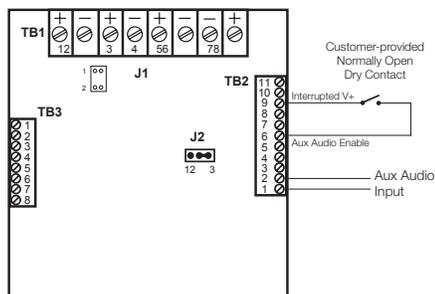
Field wiring connections
