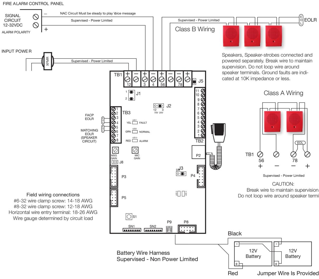
**Field wiring connections**
