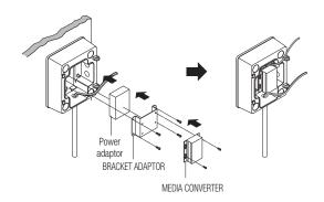
9. Pull the cable out through the door and wall mount and mount the door on the housing. (Return the locking lever to its original position and check that the hinge is properly attached to the housing.)
