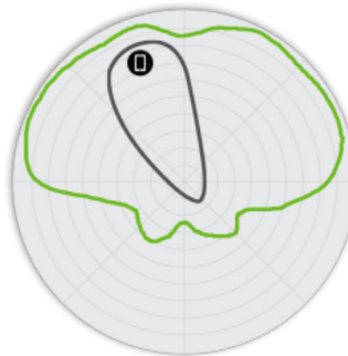
Figure 4. A750 2.4GHz Elevation Antenna Patterns
