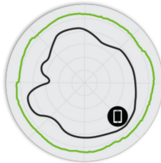
Figure 3. A750 5GHz AzimuthAntenna Patterns
