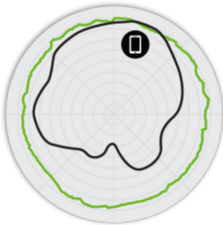
Figure 2. A750 2.4GHz AzimuthAntenna Patterns
