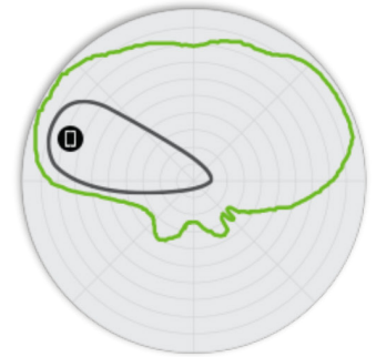
Figure 5. A750 5GHz Elevation Antenna Patterns
